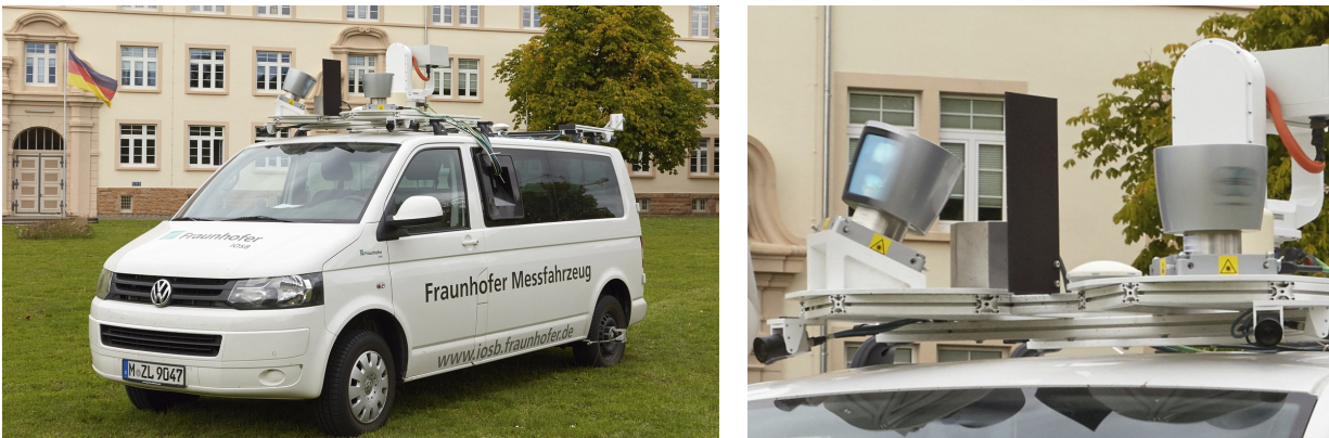
Figure 5: IOSB’s sensor vehicle MODISSA (left), and detail view of the two Velodyne HDL-64E laser scanners (right).
